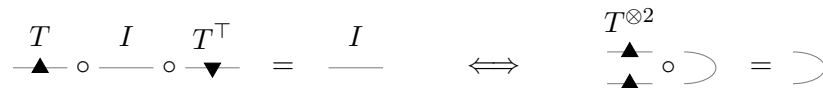
Figure 2.3: Illustrating Proposition 2.4.1. Pivoting the lower dangling edge between left and right flips the T on this edge, transposing it.
